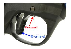
Overtravel screw (the green nylon-tipped screw): This screw eliminates the excessive rearward movement of the trigger *after* the pistol has already fired. Use your allen wrench and turn it clockwise until your trigger feels good to you and it still allows the sear to reset. If the pistol won't dry fire, back the screw out counterclockwise until it is able to.
