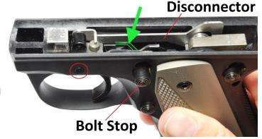
from being pushed out by engaging a small slot on one side of the pin.
