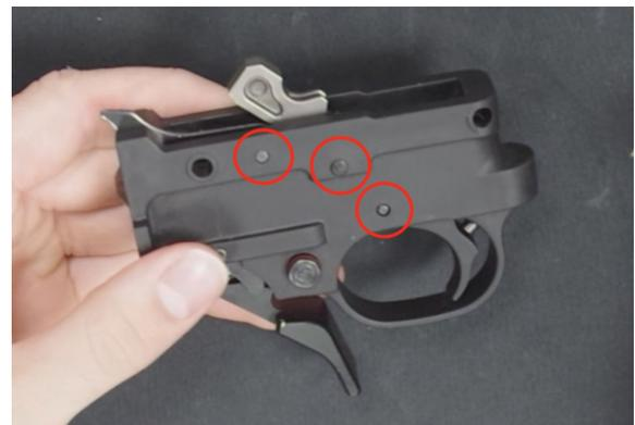
3. Punch out the pin that holds the stock disconnecter in the trigger shoe. Put the new TANDEM KROSS disconnecter into the trigger shoe as shown and replace the pin.
