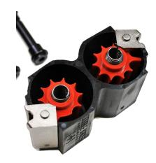
4. Snap on the back side of the TANDEMKROSS 10/22 Double Kross Housing. This will line up with the small studs on the metal feed lips and the centers of the internal rotary components. The hex cutouts are facing out.
