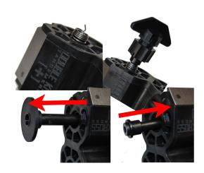
7. Turn the Hex Nut 1 and ½ Turns with the wing nut holder. Once the spring tension is high enough the hex nut will start to pull into the housing. Press the hex nut it into the housing firmly. Tighten the other end of the bolt with the Allen Key. Repeat Steps 5 and 6 for 2nd spring unit.
