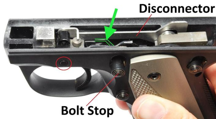
3. Using a small punch or tool, press down on the Trigger Pivot Retainer as close to the Trigger Pivot Pin as possible while simultaneously pushing the Trigger Pivot Pin out of the frame from either direction. Depending on the variable tolerances of your individual firearm, it may be easier to press the retainer down from between the plastic frame's sidewall and disconnecter lever or between the disconnecter lever and trigger.
