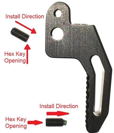
**Before installing the trigger into the gun, install the included set screws into the trigger. This must be done before putting the trigger in the gun. The pre-travel set screw is easiest to install from the top with the hex opening in**
