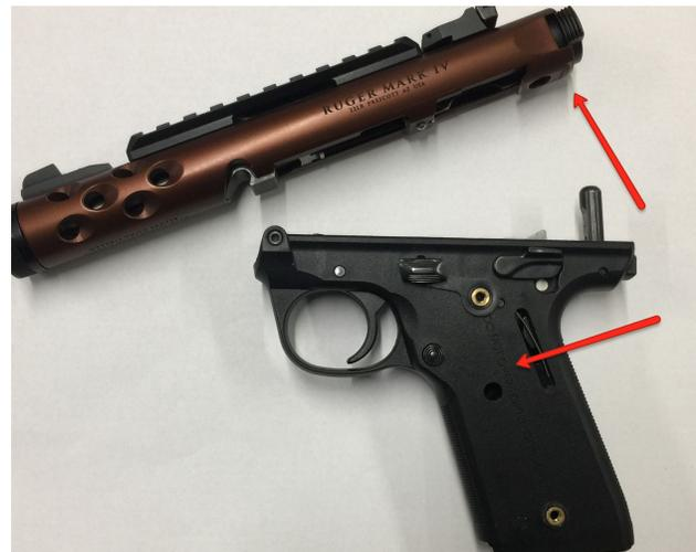
3. Uncock the pistol. Place an unloaded magazine into the pistol, put the pistol on fire and pull the trigger. Alternatively you can lift the magazine safety with a tool and pull the trigger.
