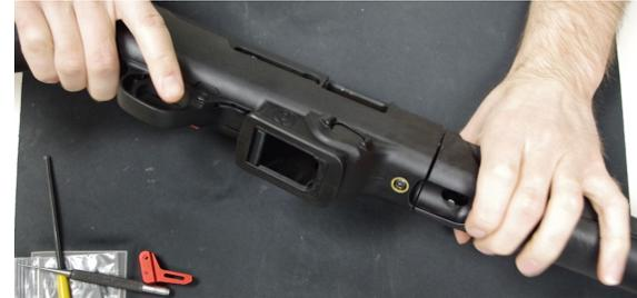
2. Loosen the two stock screws using a 5/32” allen wrench. One is in front of the mag well, one is behind the trigger guard. The screws are captive and do not need to be removed all the way. Just loosen enough so that receiver can be separated from stock. Be aware that the dowel pins that hold in the trigger housing have a tendency to fall out thus this procedure is best done in a controlled environment.
