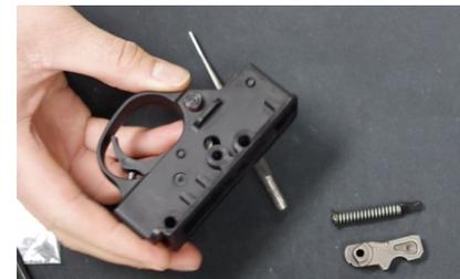
4. With the hammer disengaged from the sear, the hammer pin can easily be pushed out of the trigger housing. Remove hammer.
