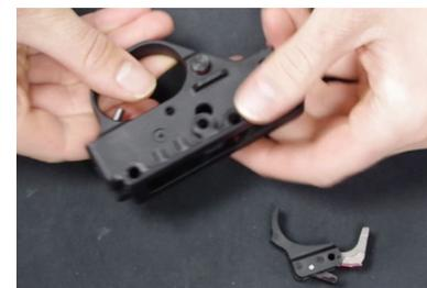
6. Remove 3/32” pin from trigger to release disconnecter, sear, and sear spring. Take care not to misplace sear spring. Replacement sear springs are available from TandemKross.
