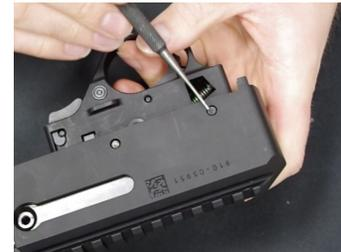
3. Push two dowel pins out of receiver to release trigger housing using allen wrench. Drop trigger housing from receiver. Release hammer from sear by turning off safety and pulling trigger. Control the drop of hammer using other hand. Remove main spring sub-assembly.
