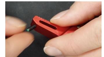
9. Hold the trigger housing so that the trigger return spring and plunger are held in by gravity as shown. Insert trigger sub-assembly into trigger housing. Align the slave pin and dowel pin through the hole in the trigger housing. Push the slave pin out with the 1/8 trigger pivot pin. Squeeze the trigger to verify smooth operation.
