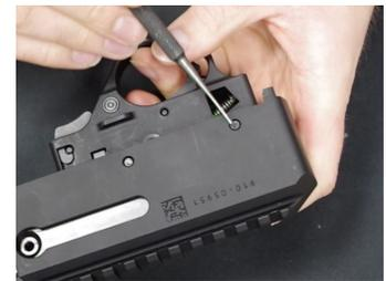
4. With the hammer disengaged from the sear, the hammer pin can easily be pushed out of the trigger housing. Remove the hammer.
