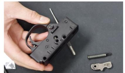
5. Remove the trigger sub-assembly pivot pin. Remove trigger sub-assembly. The trigger return spring and plunger can stay in the trigger housing.
