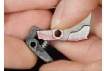
Set them back into the trigger and replace the smallest pin. Install the slave pin through the trigger and the sear. The trigger sub-assembly is now ready to be installed in the trigger housing
