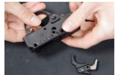
6. Remove 3/32" pin from trigger to release disconnecter, sear, and sear spring. Take care not to misplace sear spring. Replacement sear springs are available from Tandemkross.
