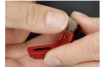
8. Take the nylon tipped screw out of the hardware bag and screw it metal end first into the hole on the rear face of the trigger. This will be your overtravel adjustment screw. You can use the included allen wrench to adjust it to your liking once the install is done.
