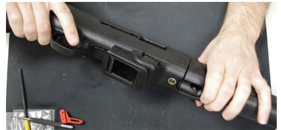
3. Push the two dowel pins out of the receiver to release trigger housing using an allen wrench. Drop the trigger housing from the receiver. Release the hammer from the sear by turning off safety and pulling the trigger. Control the drop of the hammer using your other hand. Remove the main spring sub-assembly.
