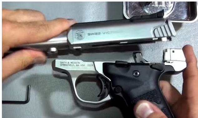
2. Insert the empty magazine and pull the trigger to drop the hammer. Eject the magazine, then remove both grip panels, starting with the RIGHT grip. Take care to not lose the magazine release and spring which is located under this grip panel. Remove the magazine release and spring and bolt stop lever and set them aside.
