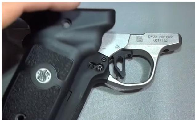
3. Using forceps or pliers, remove the spring next to safety lever and set it aside.
