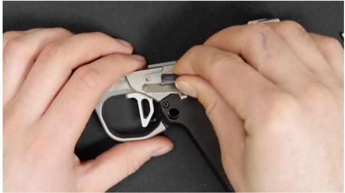
9. Cock the hammer. If the hammer refuses to pull back, it means the hammer strut is misaligned with the main spring. Push the hammer all the way forward, then pull it back, and it should align itself correctly. Test the functionality of the safety and trigger. If both work as expected, cock the hammer again and replace the barrel. **Note: the barrel will not reattach is the hammer is not cocked.**
