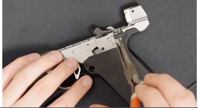
4. Push the hammer pin out of the gun from the left side and set it aside.
