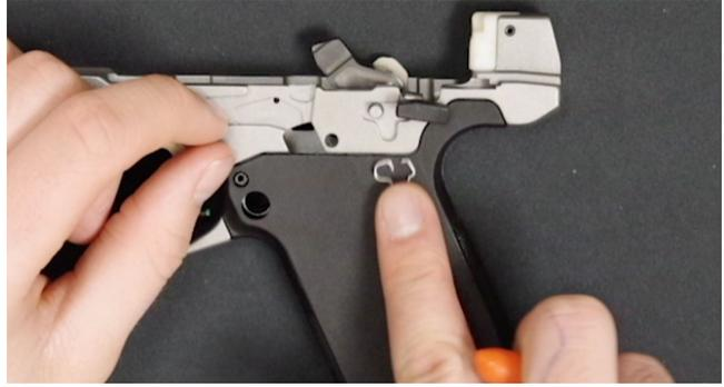
8. Replace the bolt stop lever, the left grip plate, the magazine release and spring, and the right side grip plate.
