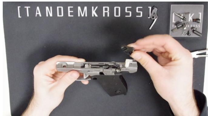
6. Apply gentle downward and forward pressure to the hammer so that the holes through the frame, safety, hammer, and trigger bar all line up, then re-insert the hammer pin from the right side. Tip: Rotate the top of the hammer toward the front of the gun to assist with hole alignment.
