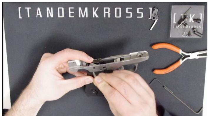
7. Replace the spring in front of the safety. To avoid scratching the frame of your gun, use a brass punch to compress the spring into it's space.
