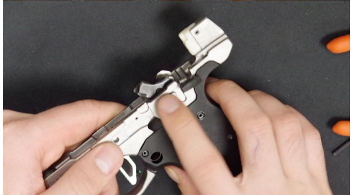
5. Lift the factory hammer out of the gun and set it aside, then place the Thunder Hammer in the gun where the factory hammer was. The flat face of the hammer should be facing the front of the gun, and the strut should be toward the back of the gun and pointing down towards the main spring.
