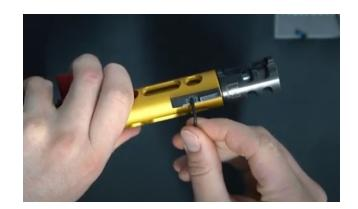
Position TANDEMKROSS front sight on the barrel and hold it in place as you screw in the included Torx screw with the included Torx wrench. The Torx screw may be too long to use with bull barrel models - either use the stock screw or sand/file down the length of the Torx screw to fit.
